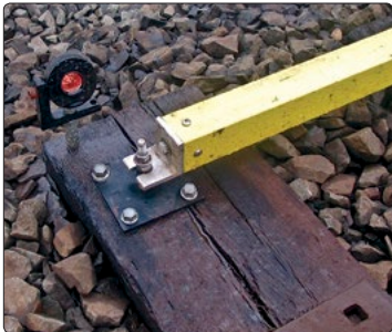
● MEMS Tilt Beam mounting attachment (with optional survey target).
